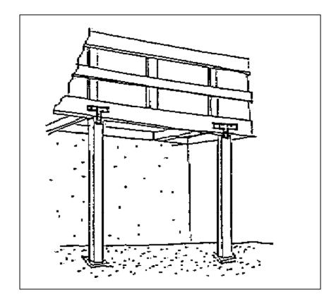
Provide post anchors at bottom of posts in crawl spaces rather than just resting on concrete pad (i.e., patio decks, stairs). Use metal connectors at post and beam connections in garages, decks, porches and basements.
